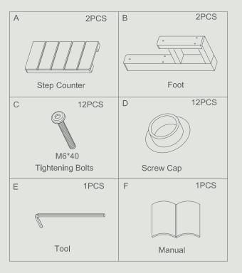
3. Place the step counter on the foot and fix it by using the tightening bolts and screw caps. It can be helpful to turn the foot upside down when doing so.
