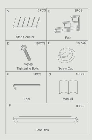
3. Place the step counter on the foot and fix it by using the tightening bolts and screw caps. It can be helpful to turn the foot upside down when doing so.
