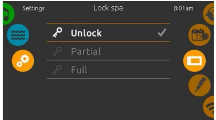
When locking the keypad, you will be asked to select a four-digit code. The same code will be needed to unlock the keypad. This will happen each time you lock the spa.
