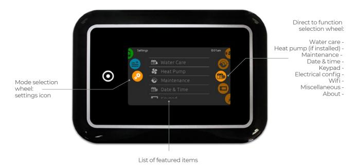
To select the settings mode, slide the left wheel up or down until the settings icon menu is highlighted in the middle. On the settings page, you can access the following:
